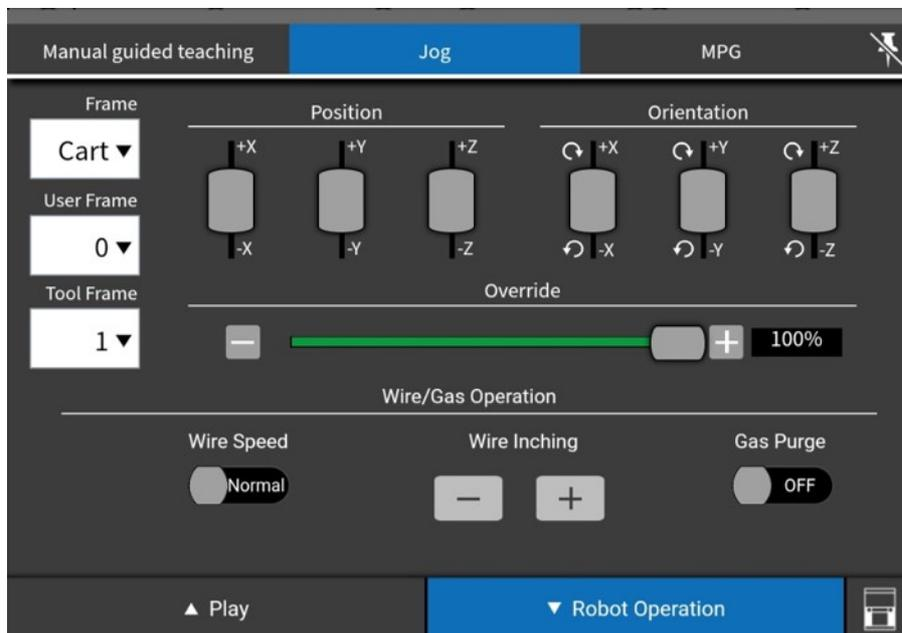
Fig. 9.5.3 The Robot Operation panel for arc welding
