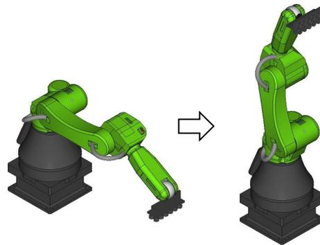
4 Insert CALL commands to call “CRDIAG(parameter)” before and after each movements. CRDIAG is KAREL program installed by default.
