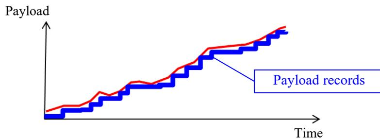
During normal operation, recorded payload is canceled from payload detected by sensor.
