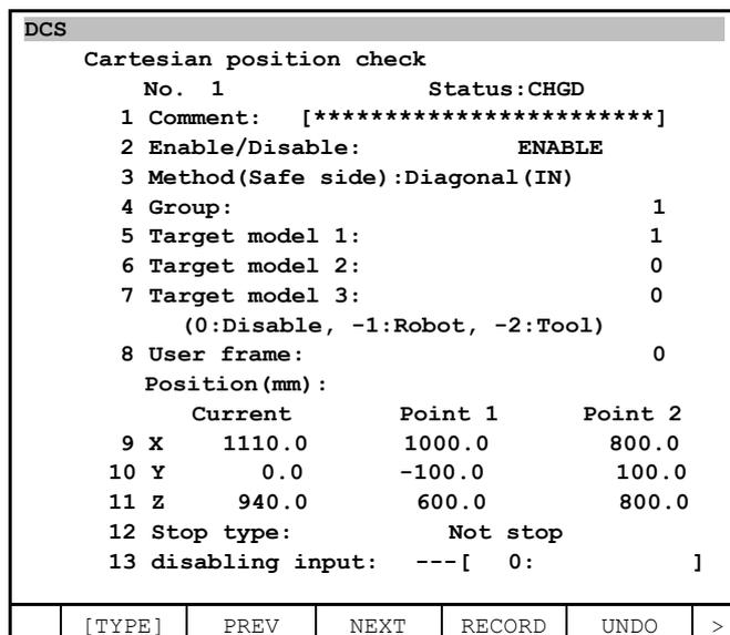
8. Apply to DCS parameter. Refer to Dual Check Safety Function OPERATOR'S MANUAL (B-83184EN), Chapter of OVERVIEW, Section of APPLY TO DCS PARAMETER.
