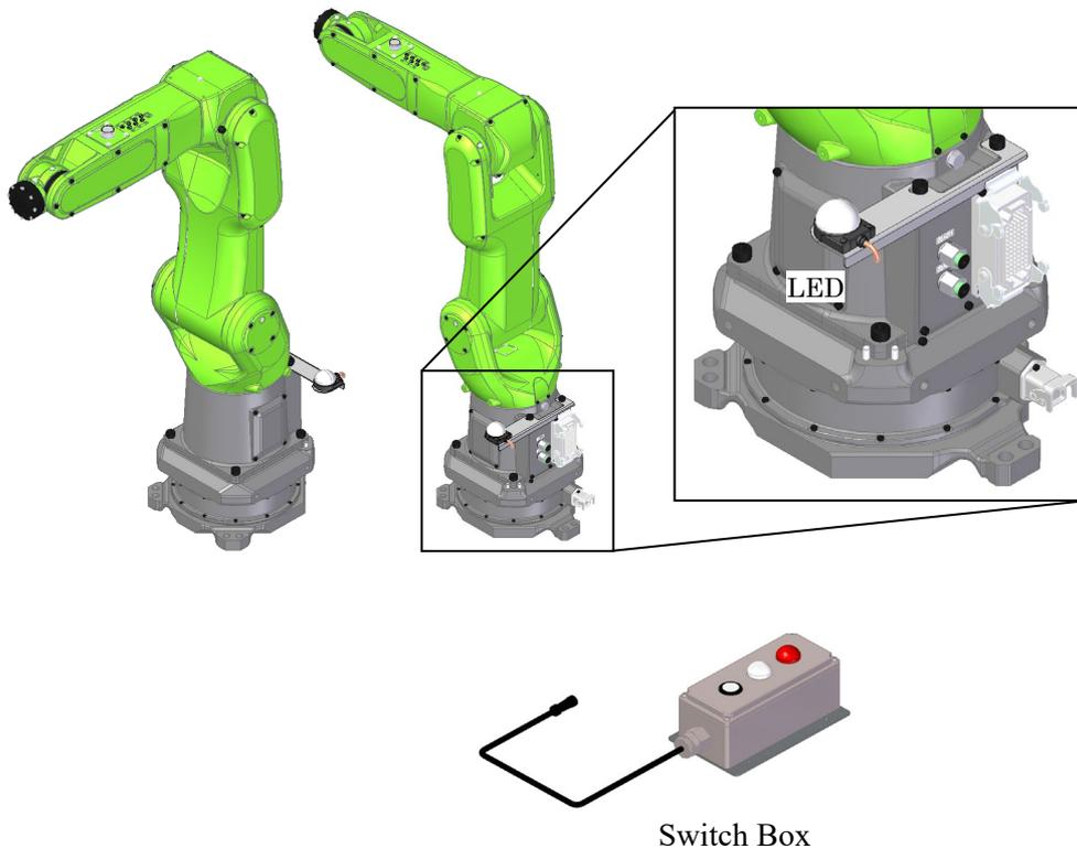
By default, these LED and button are not assigned to any function. The following is the example to set up the LED and Button.
