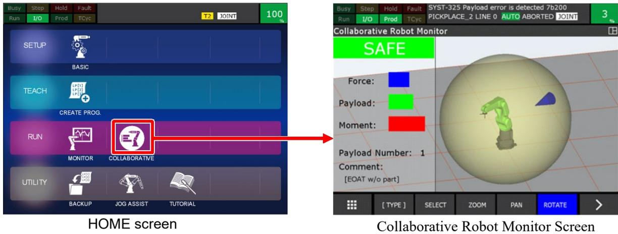
Fig. 8.4(a) Screen display flow (Collaborative Robot Monitor)
