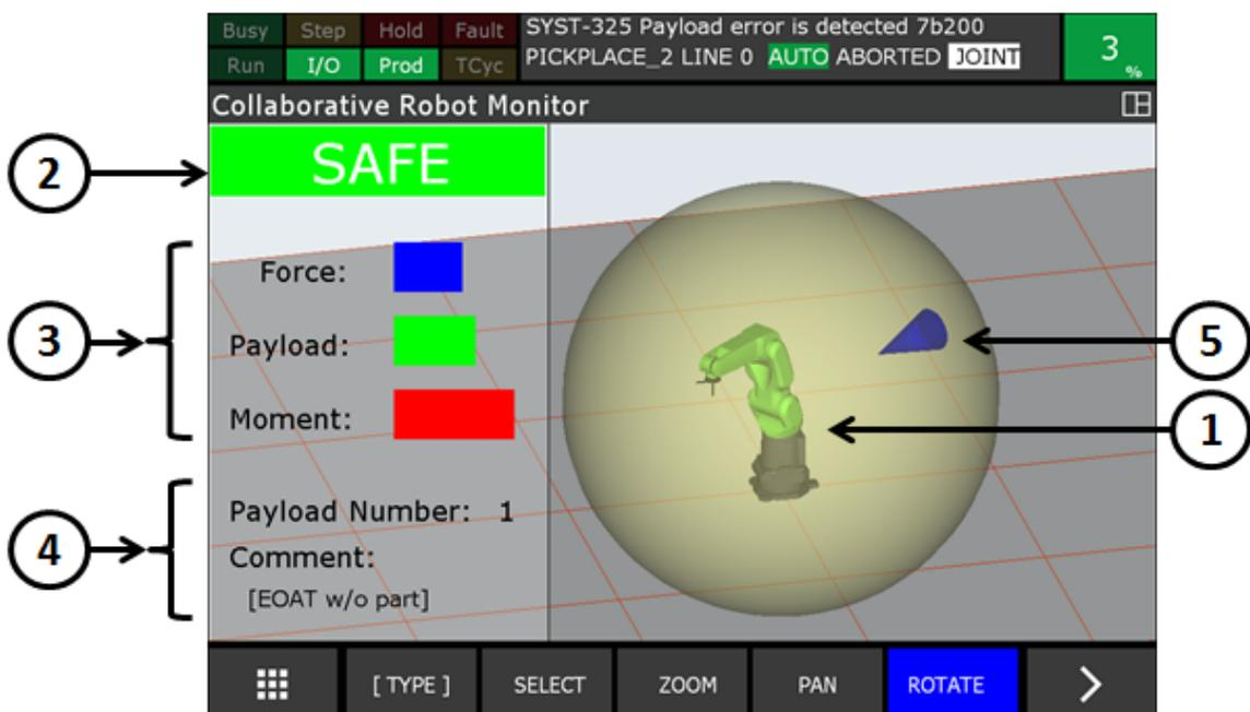
Fig. 8.4.1(a) Information on Collaborative Robot Monitor screen
