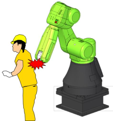
After a contact stop, the robot cannot move until the intensity of the external force becomes low.
