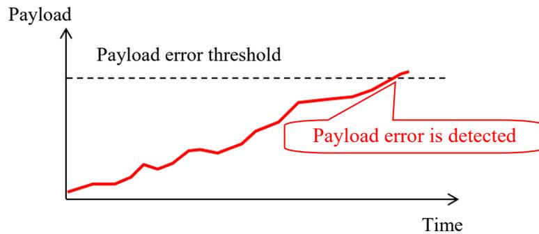
This function cancels an external payload as such system. Firstly, move the robot in RECORD mode, and Payload is recorded at constant intervals.
