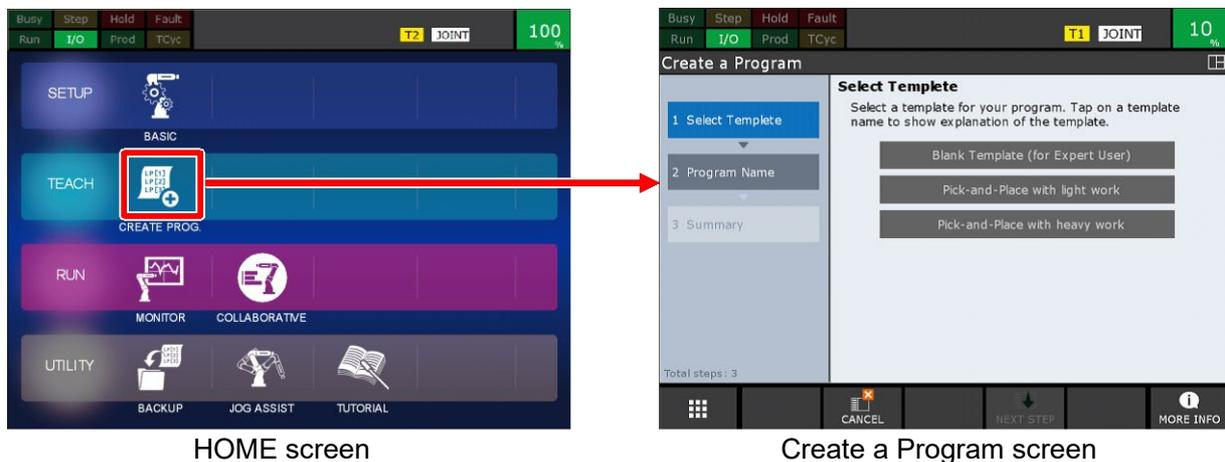
Fig.8.3(a) Screen display flow (when there are no programs)
