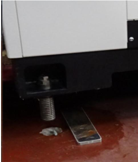
Figure 3.16. Position of the 8mm level plates
