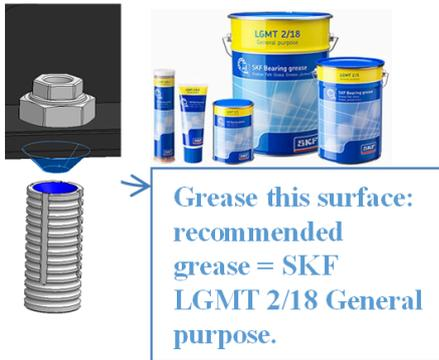
Figure 3.6. Grease in the conical anchors
