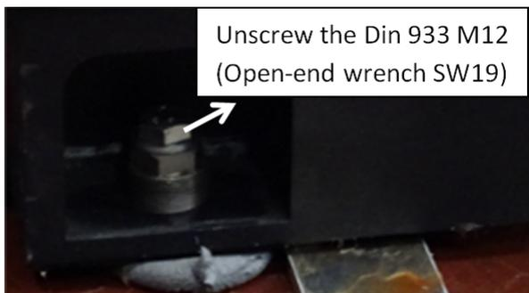
Figure 3.18. Loose the anchor screws
