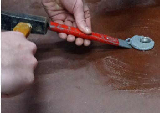
Figure 3.19. Cleaning with hammer and chisel
